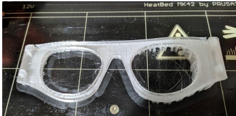
Fig. 7 - Front view of the 3D printed Neuroglass prototype.
