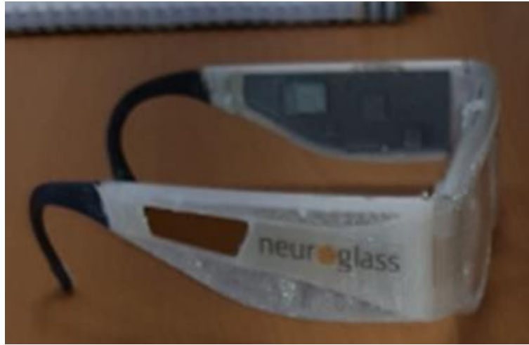
Fig. 5 - Side view of the Neuroglass with a detail of the slots for the electronic circuits.
