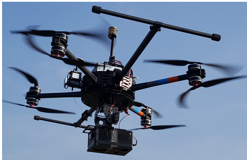
Figure 1. UAV with a box containing devices for remote sensing applications.
