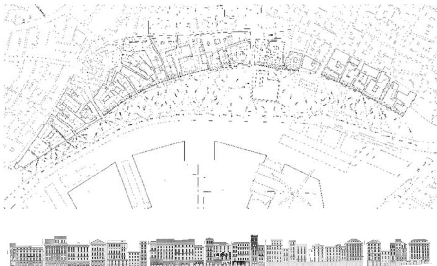
Fig. 03 : Analog Restitution of the planimetric and altimetric survey of the seafront divided into 31 lots. Direct and indirect method of trilateration and conjectural survey by G. Pellegrini
