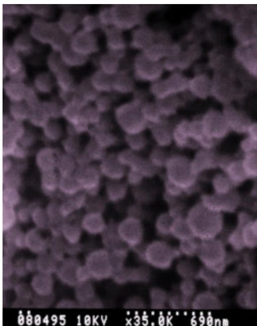
Microparticles of polyhemoglobin encapsulated in gelatin. Images obtained by Scanning Electron Microscopy. Magnification of 35,000x. Resolution of 690 nm.
