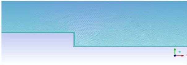
Figure 3. Unstructured mesh detail for the backward facing step
