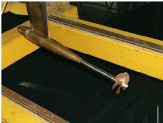
Figure 19 Towing tank open water test set-up
