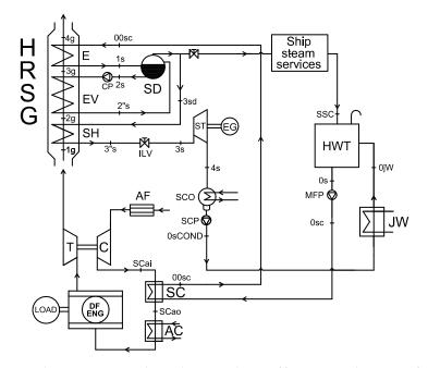
**Figure 3.** WHR single-pressure superheated-steam plant. *Abbreviations;* the same of Figure 2 with additions; SH: superheater; 1g: superheater gas inlet; 3"s: superheater steam outlet.
