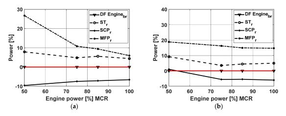
**Figure 8.** Engine and WHR plant components: power versus engine load with an engine powered by (a) NG or (b) HFO.
