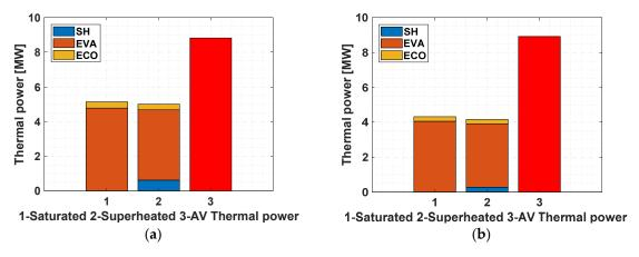
**Figure 5.** Engine exhaust gas thermal power (3) and thermal power recovered by (1) saturated- and (2) superheated-steam plant heat exchangers: E, EV, and SH, with an engine powered by (**a**) NG or (**b**) HFO.
