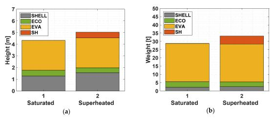
Figure 4. (a) Height and (b) weight of saturated- and superheated-steam HRSG plant components.
