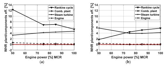
**Figure 11.** WHR plant and component-efficiency comparison versus engine load with an engine using (a) NG or (b) HFO.
