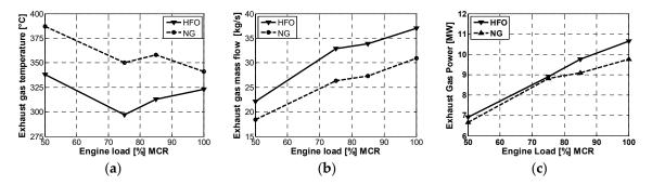
**Figure 1.** (a) Engine exhaust gas temperature, (b) mass-flow rate, and (c) thermal power versus engine load for two possible engine fuels.
