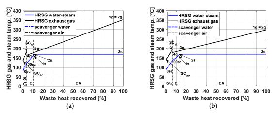
**Figure 6.** Temperature profiles along HRSG for saturated-steam plant with an engine powered by (**a**) NG or (**b**) HFO.
