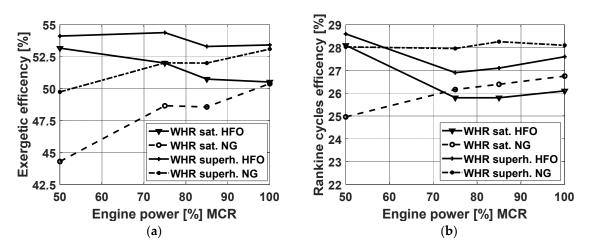
Figure 12. WHR steam-plant (a) exergetic and (b) energetic efficiency variations versus engine power.
