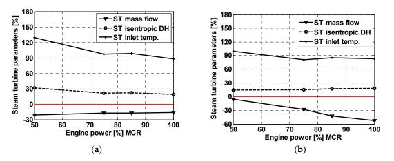
Figure 9. Steam-turbine parameters versus engine load with an engine powered by (a) NG or (b) HFO.
