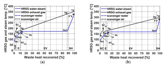
**Figure 7.** Temperature profiles along HRSG for superheated-steam plant with an engine powered.by (a) NG or (b) HFO.
