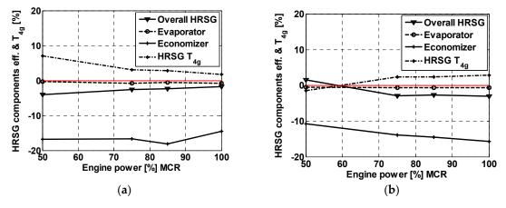
**Figure 10.** HRSG and components efficiency comparison versus engine load with an engine powered by (**a**) NG or (**b**) HFO.
