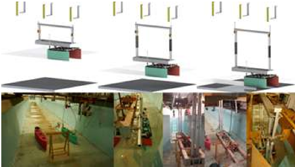
Figure 4.25: The project and the construction of the towing tank modification for the shallow water tests
