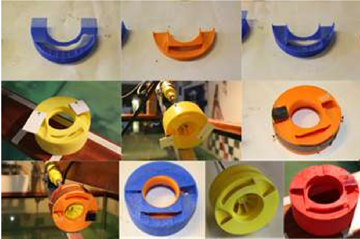
Figure 5.28: Examples of different configurations tested - Top: various central outlet designs - Middle: Tests modifying continuously the side outlets - Bottom: Various Pump-Jet configurations
