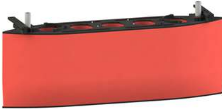
Figure 4.5: The single hull. The holes for the fast on-board systems installation can be seen.
