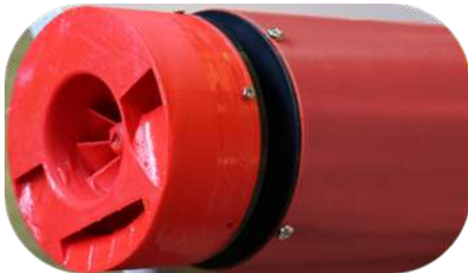
Figure 5.1: The modular Pump-Jet thruster for ASV operations in extremely shallow water.
