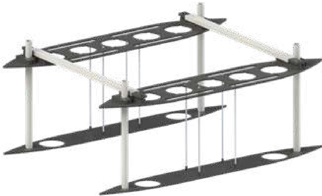
Figure 4.8: The rigid frame of SWAMP structure
