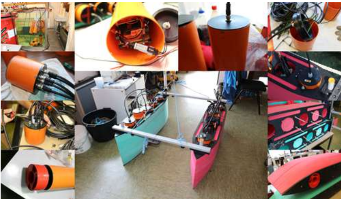
Figure 7.2: SWAMP assembly procedure and the final installation
