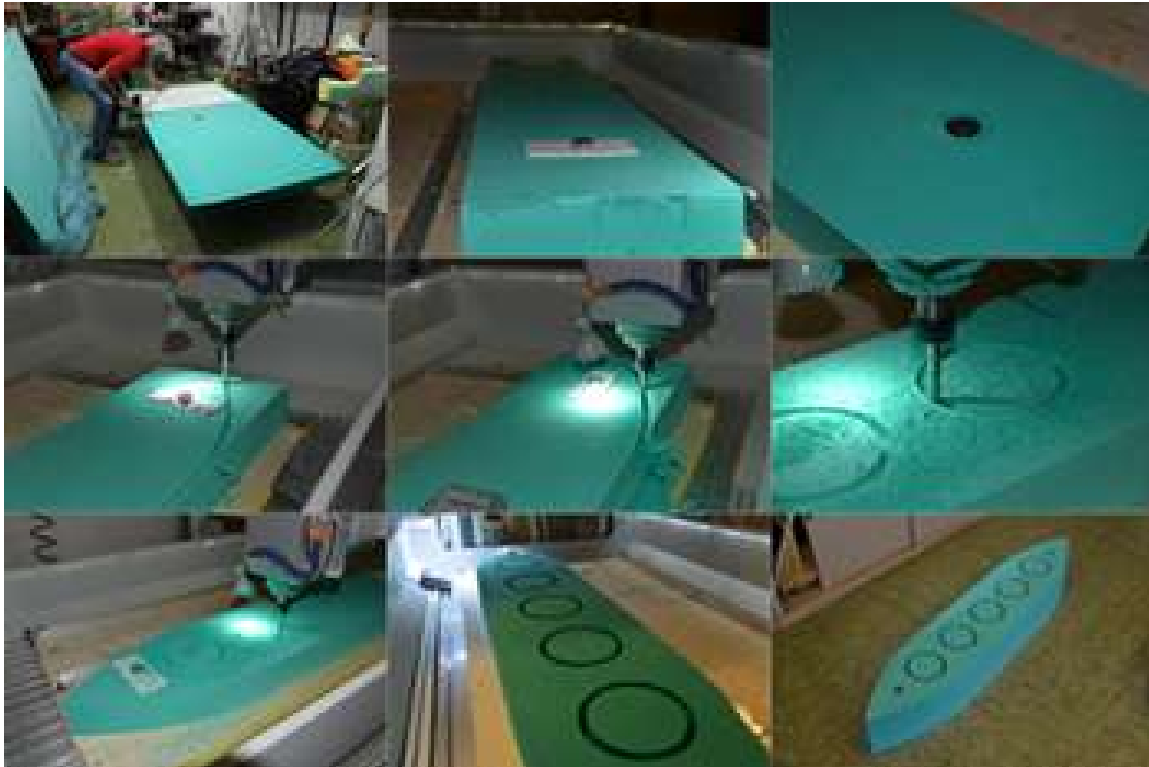
Figure 4.12: Pictures of the hull machining process
