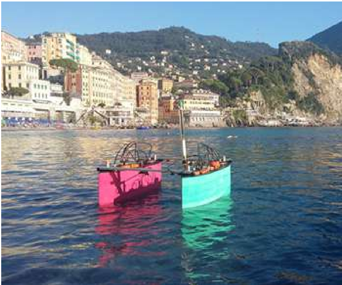
Figure 4.1: SWAMP (Shallow Water Autonomous Multipurpose Platform)
