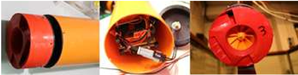
Figure 5.26: The Pump-Jet Module final layout
