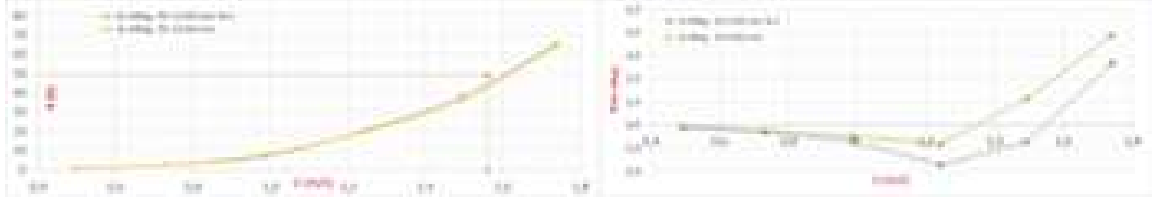
Figure 4.32: The difference in resistance and trim to static trim correction
