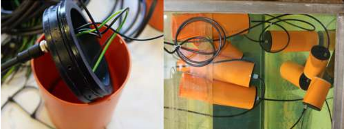
Figure 7.1: SWAMP elements water pressure tested
