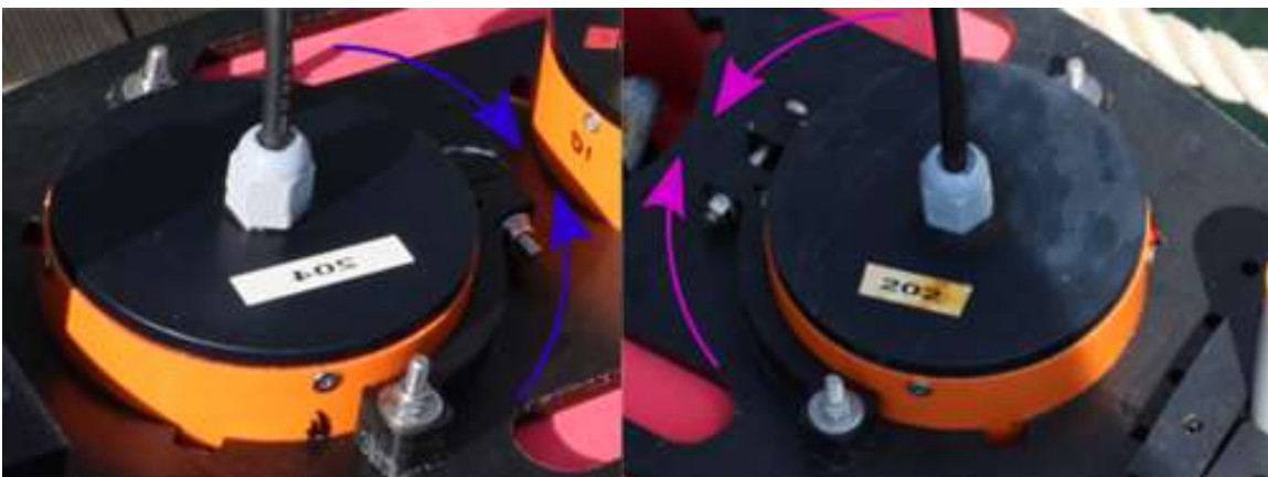
Figure 7.3: The clamp for blocking the motor's rotation
