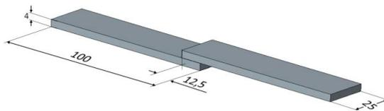
Fig. 5. Specimens dimensions.
