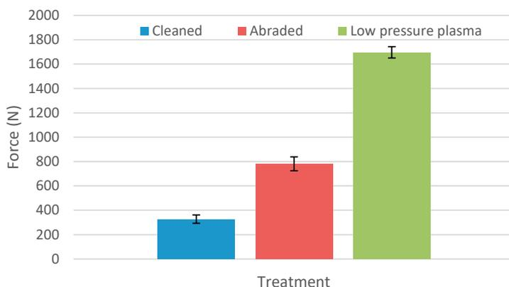
Fig. 9. Lap shear tensile test output.
