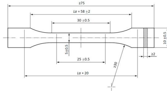
Fig. 3. Specimen dimensions.
