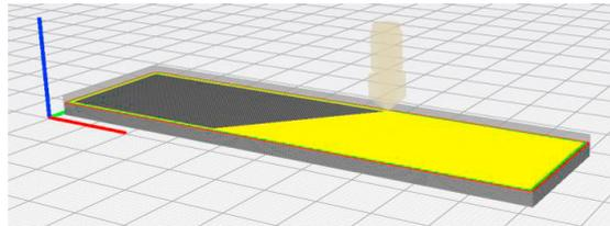
Fig. 4. Specimen positioning in the 3D printer.
