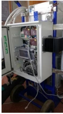
Figure 34: (a) TRT machine developed at the University of Genova, (b) Temperature profiles during the first 100 hours of the pulsated TRT experiment
