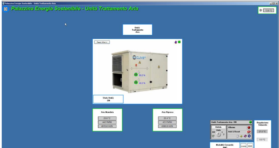
Figure 51: DESIGO page for the AHU monitoring
