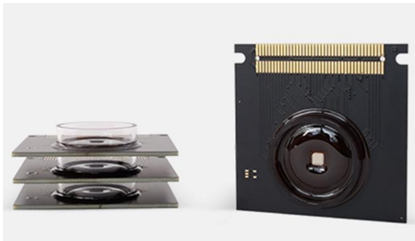
Figure 14: Example of commercially available CMOS-MEA device.
