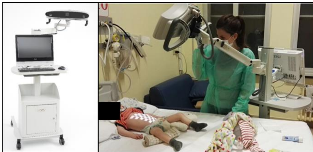
Figure 1. PneuCare Thora3DI System device and acquisition of respiratory pattern in a child with SMA type 1. SLP projects a grid of light onto the thoraco–abdominal (TA) wall of a participant. The grid is centred on the patients' xiphoid process. Changes in the grid pattern are recorded by video cameras in the scanning head.
