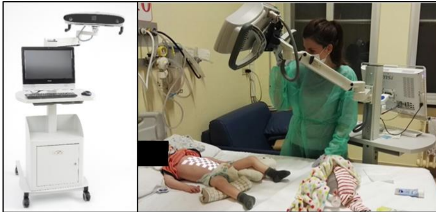
Figure 7. Structured light plethysmography PneumaCare Thora3DI® System device and acquisition of respiratory pattern in a child with SMA type 1. The PneumaCare Thora3DI® projects a light grid on the chest of the patient lying in supine position. PneumaView™ bi-dimensionally reconstructs the displacement of the thoraco-abdominal light grid.
