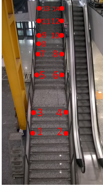
Figure 1: Positions of accelerometers on the staircase
