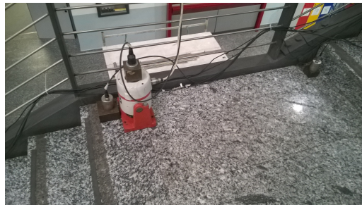
Figure 2: Source of external load: shaker moving a mass
