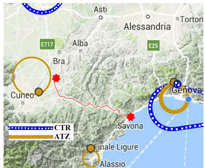
Fig. 11. Map on trafficking carried out by the drone. Brown represents the ATZ and blue the CTR.
