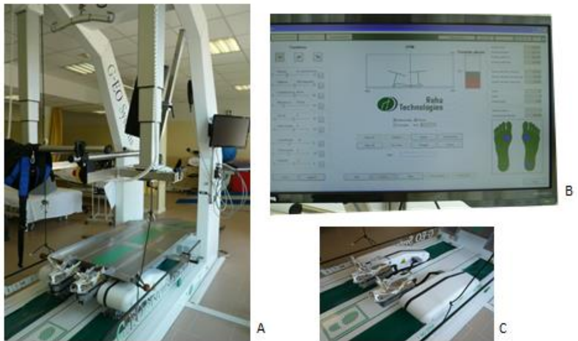
Figure1: A) G-EO system end-effector gait rehabilitation robot; B) Control panel; C) The motion mechanism of the gait robot
