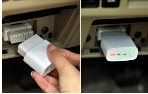
Fig. 5. OBD-II adapter plugged into car's female 16-pin OBD-II connector [50].
