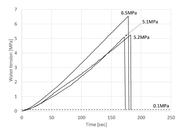
Figure 9. Evaporation tests performed with the second Ultra-High Capacity Tensiometer prototype.
