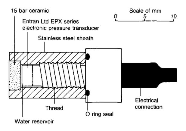
Figure 1. Imperial College High Capacity Tensiometer (Ridley and Burland, 1993).
