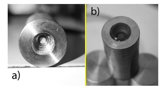
**Figure 3.** Ultra-High Capacity Tensiometer without nanoporous glass interface (a) and with a saturated nanoporous glass interface (b).
