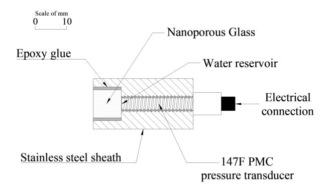
Figure 2. Proposed Ultra-High Capacity Tensiometer.
