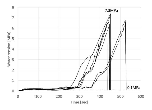
Figure 8. Evaporation tests after localized cracking of the glass interface.
