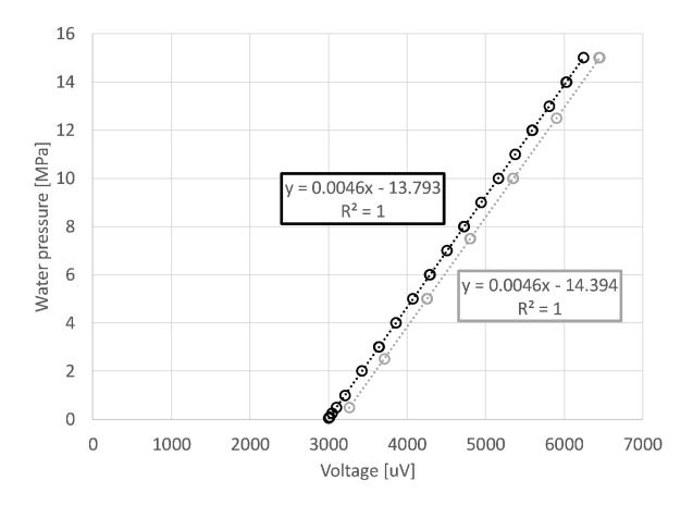
Figure 5. Initial calibration curve (black) and drifted calibration curve (grey).
