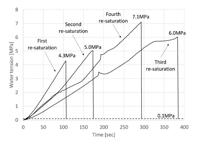
Figure 7. Evaporation tests after 72 hours re-saturation.
