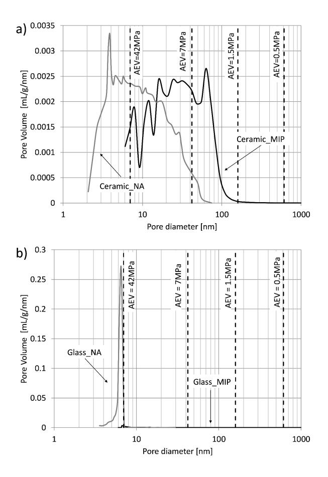
Figure 4. Pore size distribution of interfaces: a) ceramic and b) glass.
