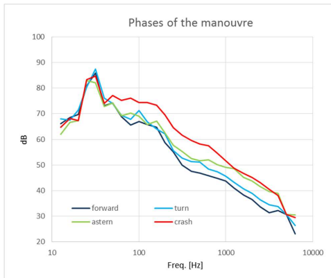
Figure 3 - Different conditions of the propulsion plant Records from position A (spectral levels, dB re 20µPa)
