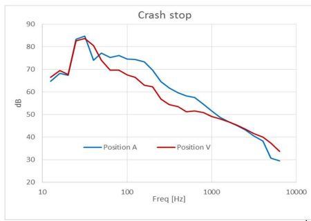
Figure 6 - same-Single phase of the manoeuvre, spectra levels surveyed in positions A and V (dB re 20µPa)
