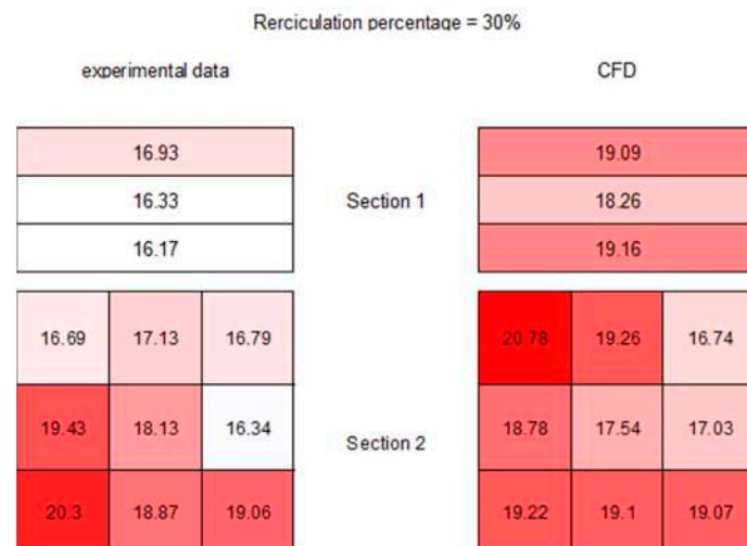
Figure 9. Comparison between experimental and CFD data for 30% WGR—O 2 mole fraction.
