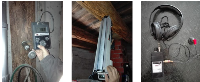
Figure 7-8-9: Non destructive tests: thermo-hygrometer, resistograph and auscultator.
