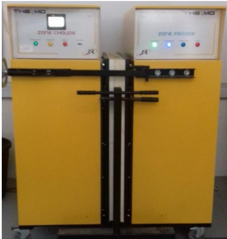
Figure 5. Testing frame containing the wall sample sealed between the hot and cold rooms of the climatic chamber.
