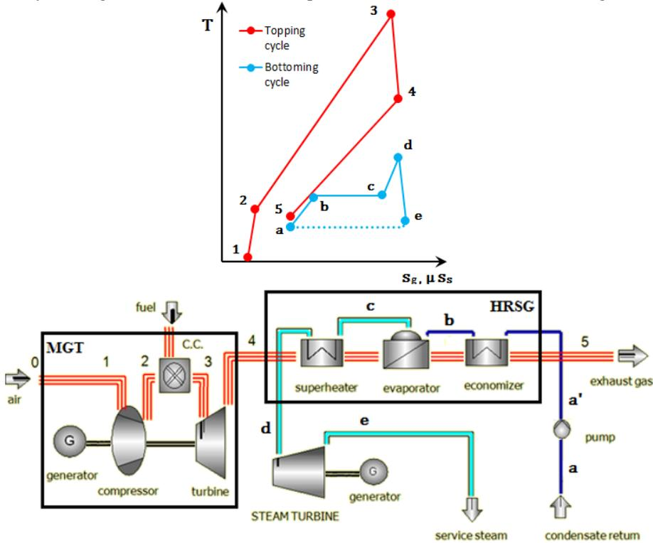
**Fig. 1.** Schematic representation of the cogeneration system
