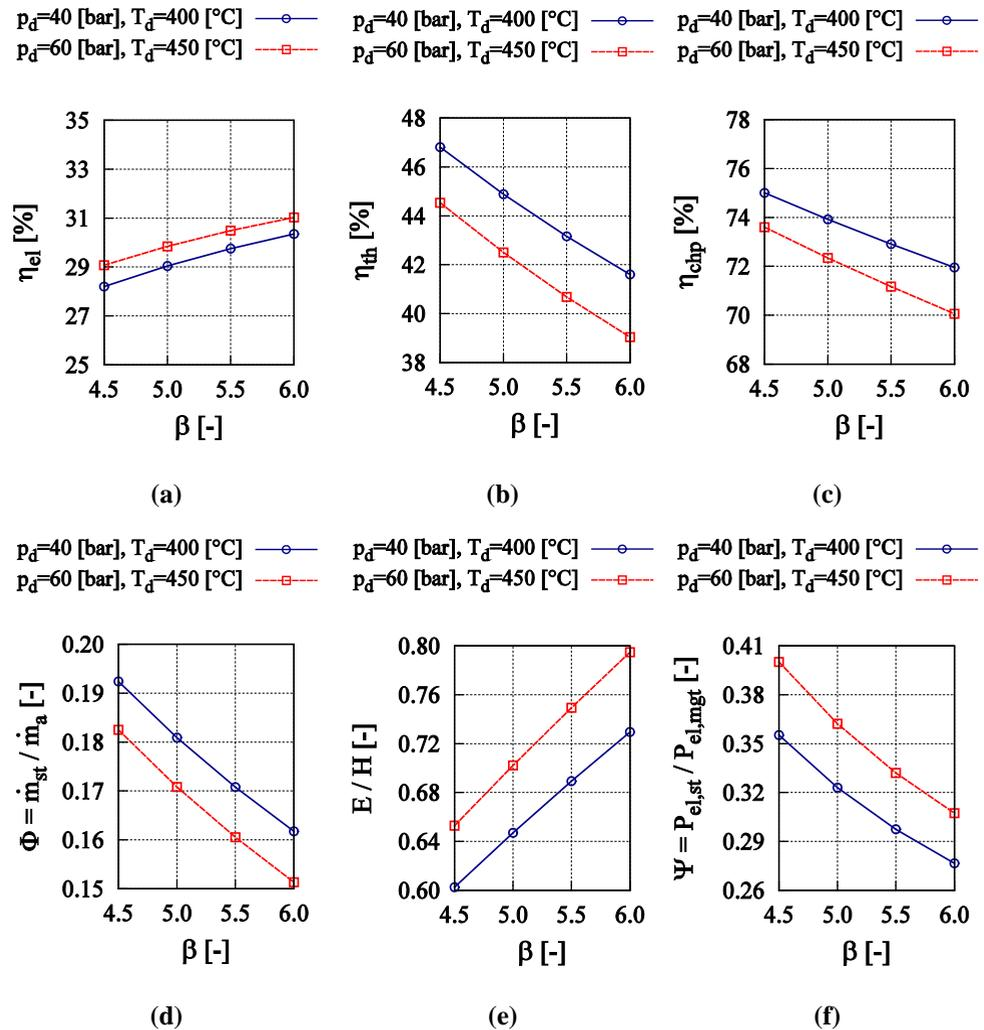
**Fig. 3.** Influence of  $\beta$  on: (a)  $\eta_{el}$ , (b)  $\eta_{th}$ , (c)  $\eta_{chp}$ , (d)  $\Phi$ , (e) E/H, (f)  $\Psi$  for steam turbine admission conditions of case A ( $p_d = 40 \text{ bar}, T_d = 400^\circ\text{C}$ ) and B ( $p_d = 60 \text{ bar}, T_d = 450^\circ\text{C}$ )
