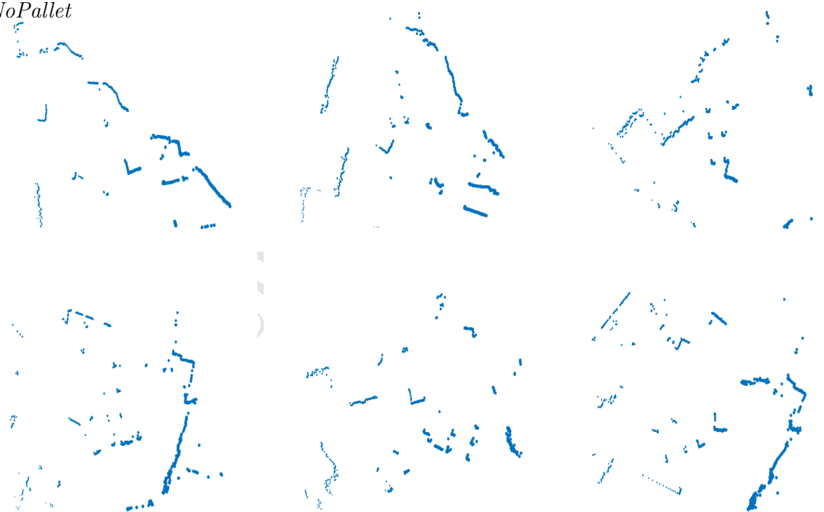
Figure 4: The dataset of real-world 2D scans represented in Cartesian coordinates: the first two rows are related to the case where a pallet is present in the environment and the operating face is free, whilst the last two rows represent samples of the dataset when no pallet is present or the operating face is not accessible by an autonomous forklift. The red box in the first image represent an example of region of interest, i.e., the part of the image actually where the pallet is located.
