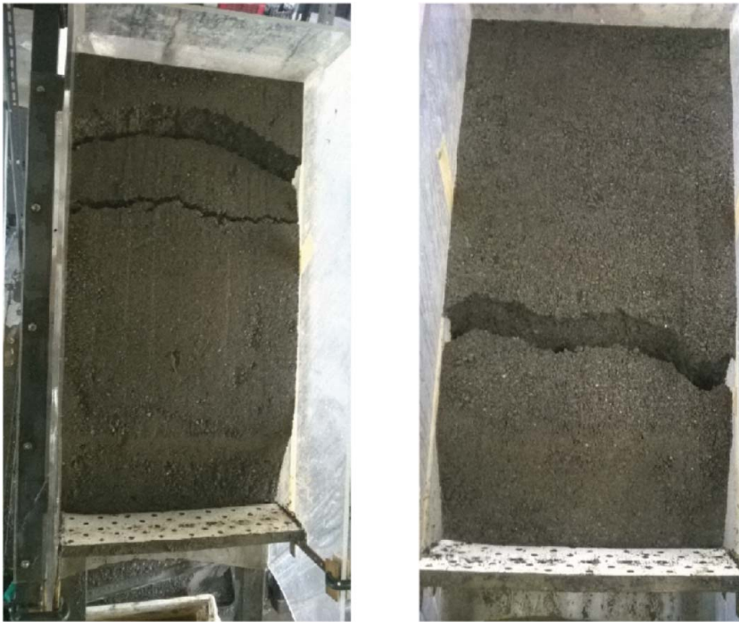
Figure 8. Post-failure images of flume tests performed on the material sampled near Giampilieri (from Montrasio et al. 2016 mod.)
