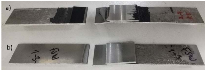
FIGURE 5: Comparison between (a) FSW and (b) FSWeld-bonded dynamic fractures
