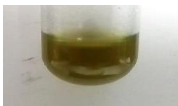
Fig. S3.1 Green coloring obtained in the FeCl 3 test performed on 9 solution
