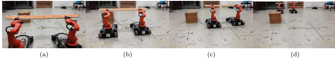
Figure 7: Obstacle avoidance experiment: snapshots of the two YouBots as they cooperatively avoid the obstacle and reach the desired final position.
