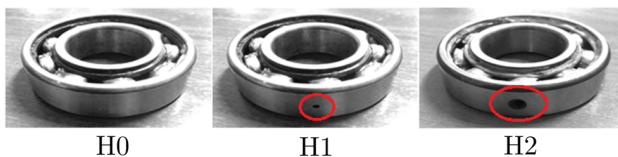
Fig. 4: Bearings Condition: New (H0), 1.6 mm hole (H1) and 5 mm hole (H2).
