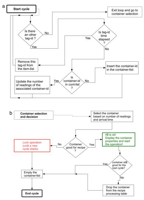
Fig. 2. Tag list processing (a) and container selection (b) flowcharts.
