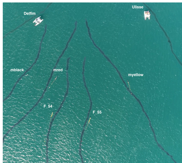
(c) Actual paths obtained during sea tests superimposed with the vehicles photographed by a drone during a trial.
