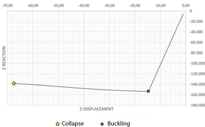
Figure 6. Collapse history: vertical displacements [mm] vs. vertical reaction [kN]
