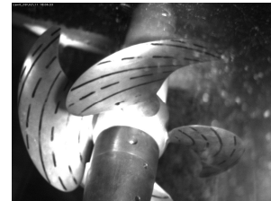
Fig. 5. Propeller 1B: Speed reduction at constant pitch, view from above
