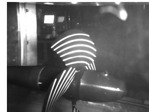
Fig. 9. Propeller 3: Speed reduction at constant pitch, view from starboard
