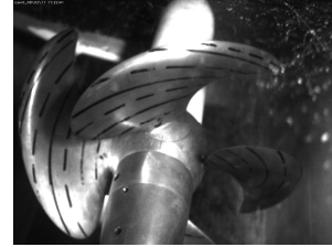
Fig. 3. Propeller 1A: Speed reduction at constant pitch, view from above
