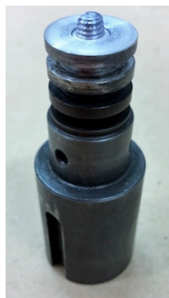
Figure 2. FSW tool used for the welding realization.
