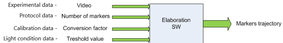
Figure B.5: Flow diagram of elaboration software
