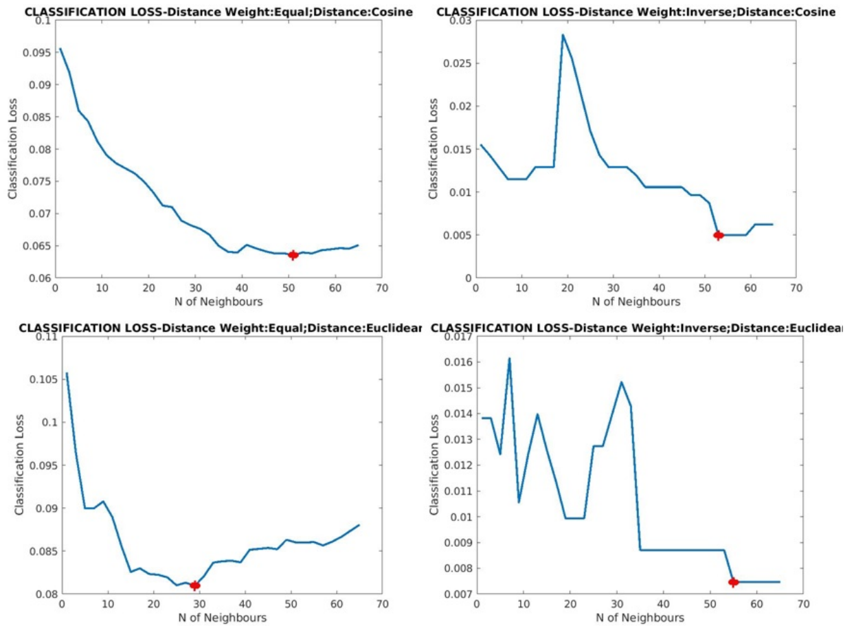
Figure 3.10: The Loss curve is used for displaying the predictive inaccuracy of the model. Dataset_1 : a) k=51 , L=0.0635 . b) k=53 , L=0.0050 c) k=29 , L=0.0810 d) k=55 , L=0.0075
