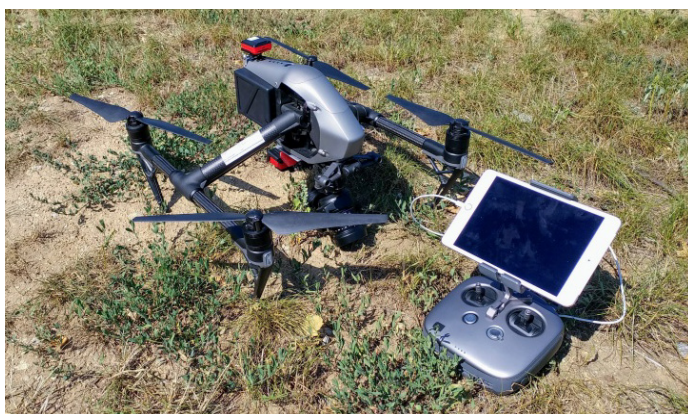
Figure 3. UAV equipped with multispectral sensor, GPS device and digital camera.
