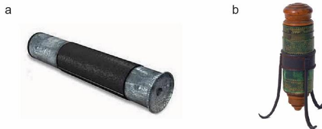
Fig. 1.2.1 The first microscopes. Reconstructions of Jansen’s (a) and Galilei’s (b) microscopes.
