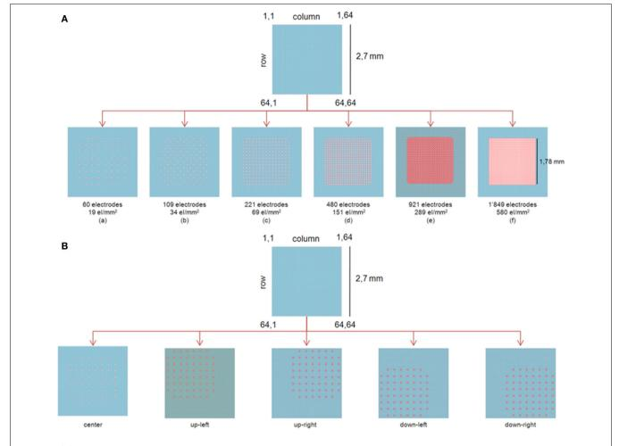
**FIGURE 2 | (A)** Layouts representation corresponding to the electrode subsets and used for analyzing the data at different spatial-scales. (top) Entire active area of an APS-MEA ( $2.7 \times 2.7 \text{ mm}^2$ ) arranged in a  $64 \times 64$  layout. (bottom) The electrode array subsets are defined by considering a constant active area of  $1.7 \times 1.7 \text{ mm}^2$ . The lowest electrode density is of 19 electrode/mm² for the 60
