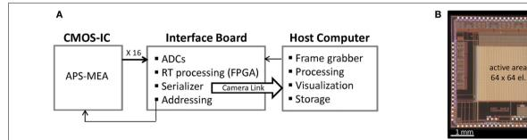
FIGURE 1 | (A) Block diagram of the acquisition platform. The high-speed communication interfaces are depicted with white arrows, whereas the low-speed ones are indicated by the black arrows. Multiplexed analogical data readout from the APS-MEA are digitized, processed and converted in a camera-link format
