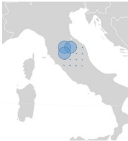
Figure 4.14: Example of grid selection of the cells. For each point of the grid, the Centre-Radius selection is performed. The radius equals the step of the grid.
