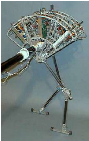
Figure 2-3: The Spring Flamingo robot used to test the virtual model (VM) control strategy.
