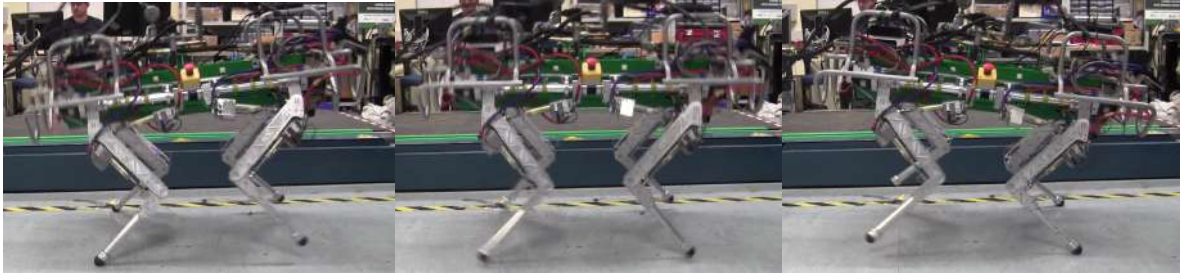
Figure 3-10: Snapshots of an experiment of self-stable bounding gait performed on the HyQ (we can see a flight phase in the middle picture). The time passing between two neighboring frames is of 70 ms.
