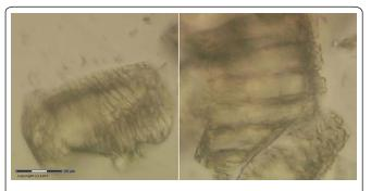
Figure 5: Domains in lysozyme Langmuir-Blodgett (10 micron) and classical (1 micron) crystals.
