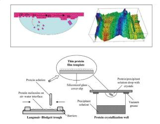
Figure 1: Pictorial scheme of the Langmuir-Blodgett (LB)-based nanocrystallography.
