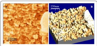
Figure 3: AFM image PGA (60 monolayers LB film) at room temperature in 2D (A) and 3D (B).
