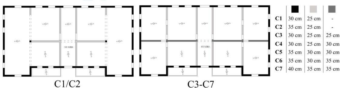
Figure 2. Structural configurations derived from the “C” type architectural configuration: a) C1 and C2 with internal r.c. beams and columns; b) C3 to C7 with internal masonry walls.
