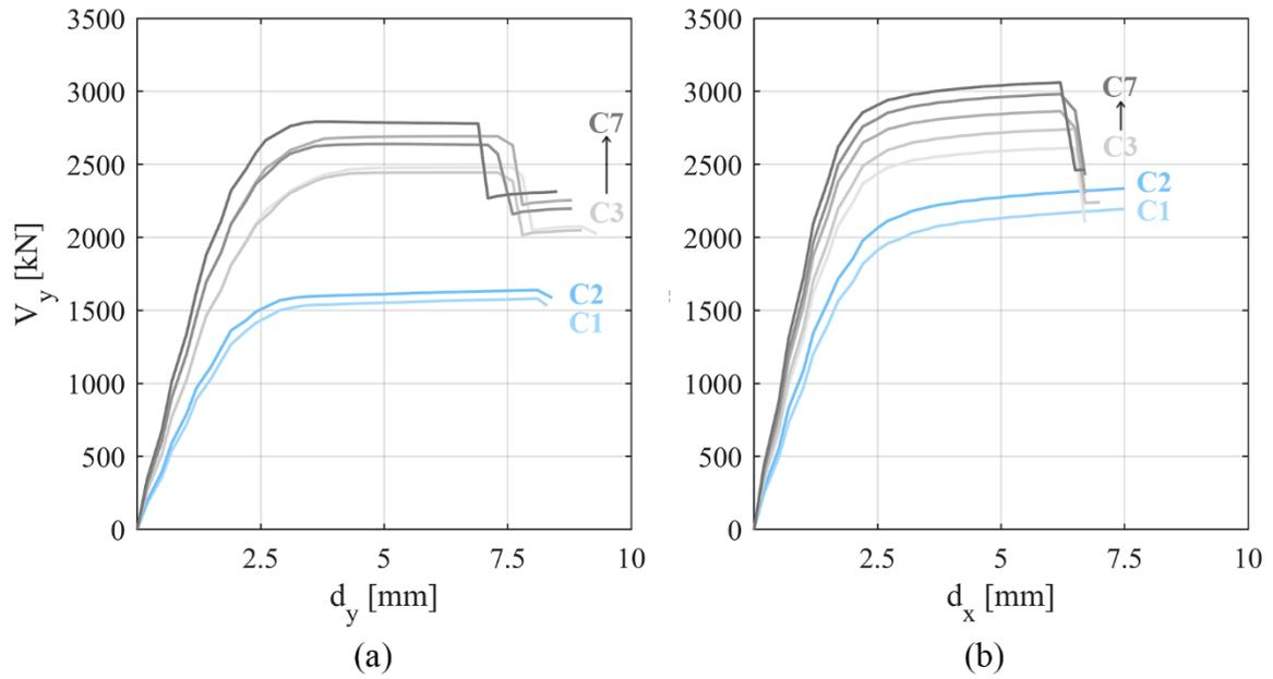
Figure 5. Pushover curves of the 3-storey “C” type configurations: (a) inverse triangular distribution and  $y$  positive direction; (b) mass-proportional distribution and  $x$  positive direction.
