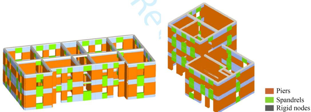
Figure 4. Examples of structural models adopted for NLSA (“C” and “I” type configurations)
