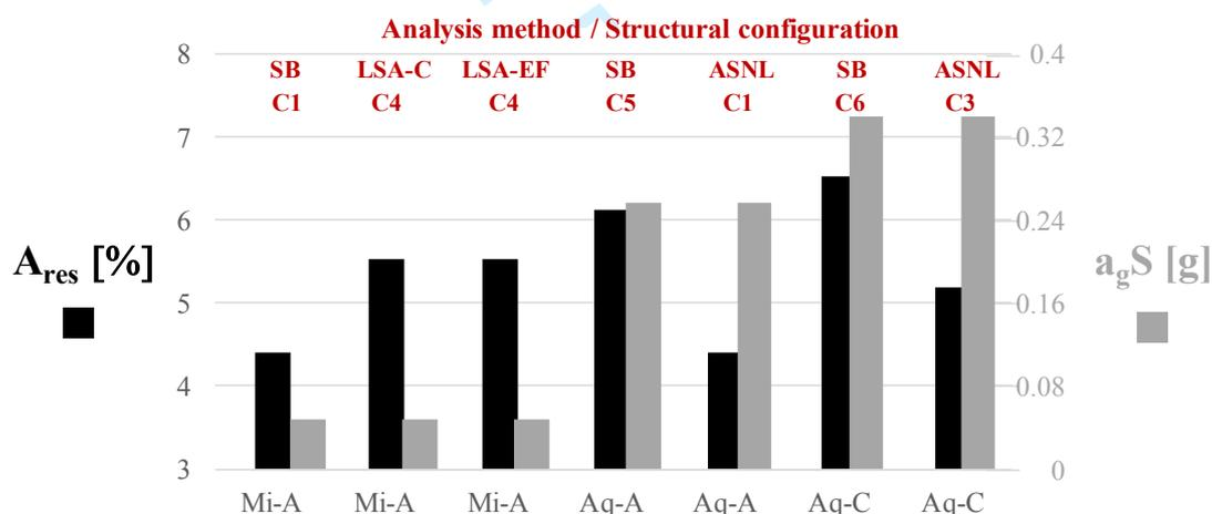
Figure 6. Overview of design outcomes for the “C” type configurations obtained with different analysis methods, highlighting the variation in the percentage of resisting masonry area over the total floor area (black) compared to seismicity (grey).
