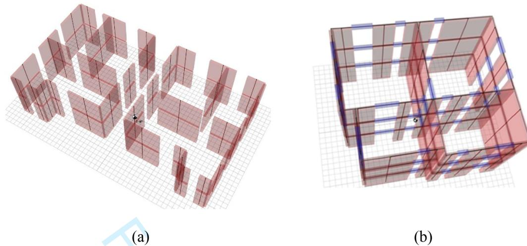
Figure 3. Examples of structural models adopted for the design according to LSA:
