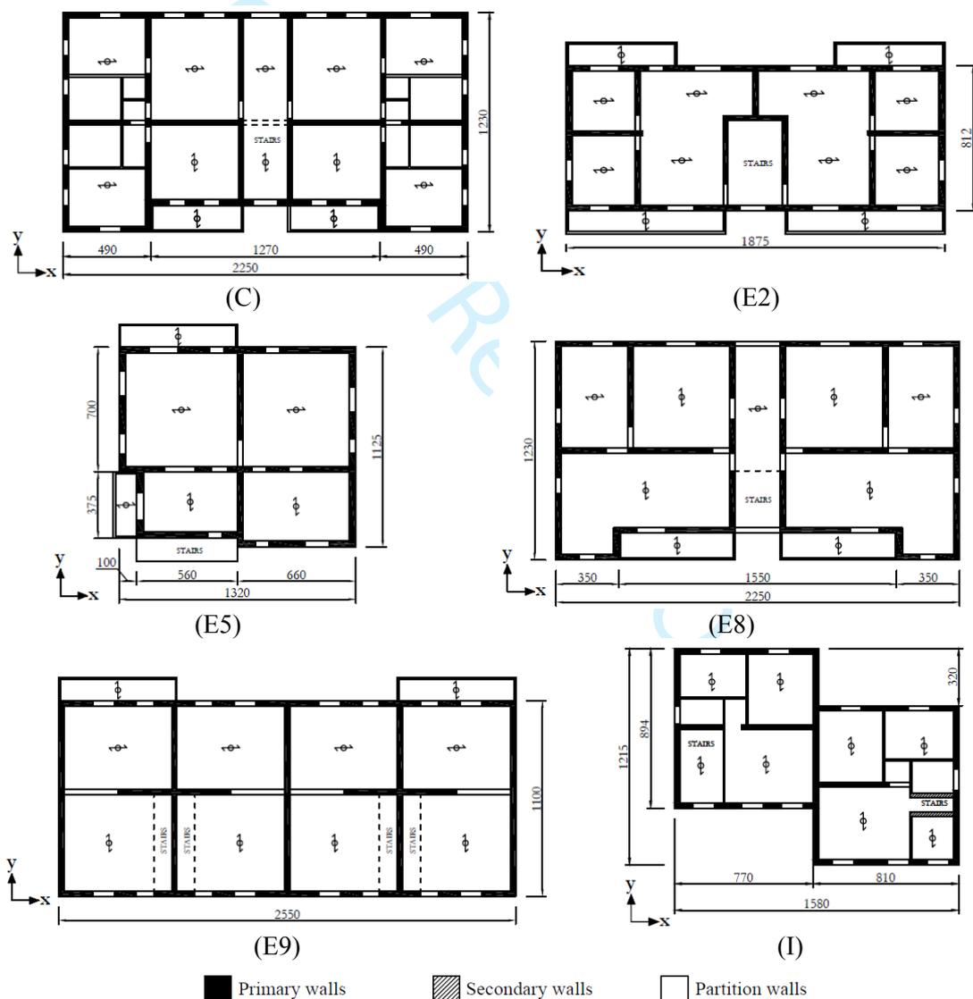
Figure 1. Selected architectural plan configurations (structural variations, namely C1 to C7, were then created starting from the reported “C” type plan, derived in turn from E8) Dimensions in the plans are in cm.
