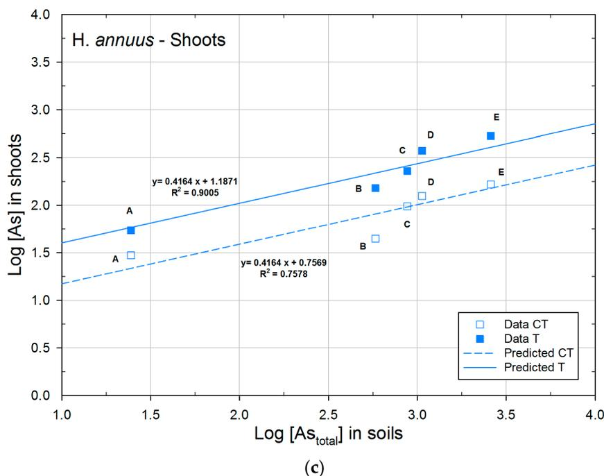
**Figure 2.** Freundlich-like equation for the shoots uptake of *B. juncea* (a), *L. albus* (b), and *H. annuus* (c) in control (CT) and phosphate treated (T) soils.
