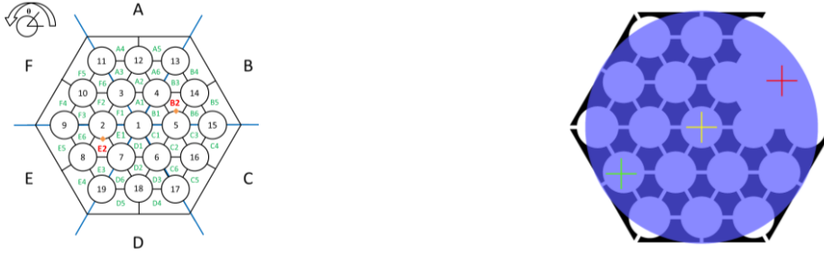
Figure 6. Sketch of the BFPS test section (edge blockage on sector B) with monitored sub-channels (red) and pins (orange) on the left. Sketch of the axial lines in the mixing region (right).
