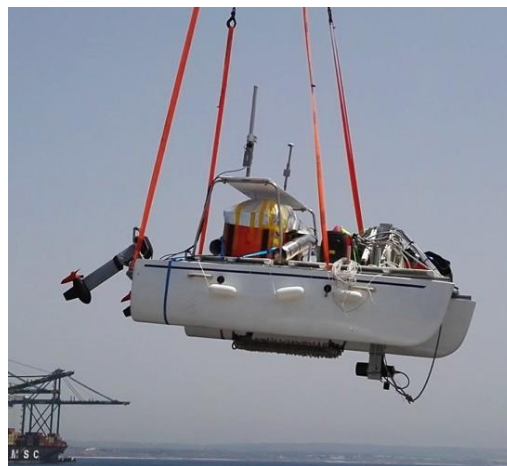
Fig. 3. ULISSE during WiMUST deployment. The acoustic sparker can be seen in the middle part. The two acoustic modem transducers can be seen near the bow.
