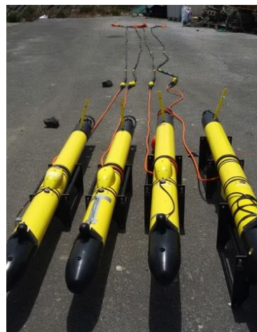
Fig. 6 Folaga AUVs towing streamers with hydrophones
