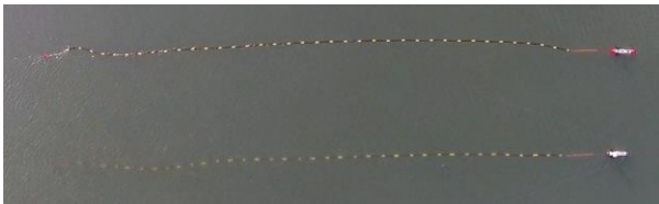
Fig. 8 Picture of Medusa AUVs towing a streamer with hydrophones
