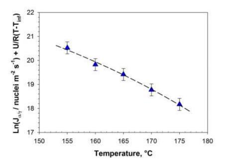
**Figure 4.** Natural logarithm of the measured cross-nucleation rate corrected for the transport term (see equation 7) as a function of crystallization temperature. Dashed black line represents the fitting of the data with equation 8.
