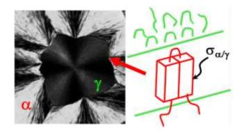
**Synopsis:** The kinetics of cross-nucleation between two polymorphs of polypivalolactone ( $\alpha$  on  $\gamma$ ) is measured for the first time as a function of crystallization temperature and successfully explained as heterogeneous secondary nucleation among different crystalline modifications.
