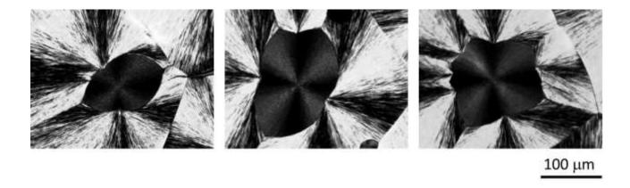
**Figure 1.** Examples of the morphologies obtained at the end of PPVL crystallization at 160 °C. Cross-nucleation of α-phase can be observed at multiple points of the  $\gamma$ -spherulites periphery.
