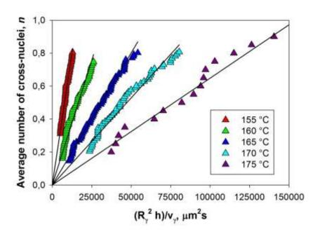
**Figure 2**. Average number of  $\alpha$ -phase cross-nuclei as a function of  $R_{\gamma}^2$  multiplied by the thickness of the sample and divided by the growth rate of the parent  $\gamma$ -spherulite. Results for different (indicated) crystallization temperatures are shown. Black lines are best fit of the data, passing through the origin of the axes.
