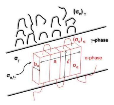
Figure 3. Schematic model for the formation of a α-secondary nucleus on the growth surface of  $\gamma$ -phase lamellar crystal. Adapted from Varga et al.<sup>16</sup>
