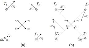
Fig. 4 – Scenarios of null contribution provided by  $b_i$  terms. a) every  $b_i$  term is null, as every  $dX_i$  vector is orthogonal to its corresponding  $u_i$ , b)  $b_i$  terms are not null but their resulting contribution to error vector e is null
