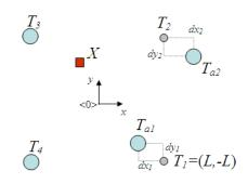
Fig. 2 –Nominal positions (grey) and actual positions (cyan) of transponders in the presence of displacements
