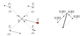
Fig. 7 – Worst-case scenario for the error contribution provided by  $c_i$  terms. The resulting vector is in bold..
