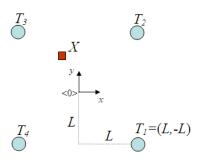
Fig. 1 – squared configuration of transponders
