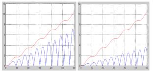
Fig. 10 - Time behaviour of the norm of e in meters (blue) and the norm of the X in hundreds of meters (red)
