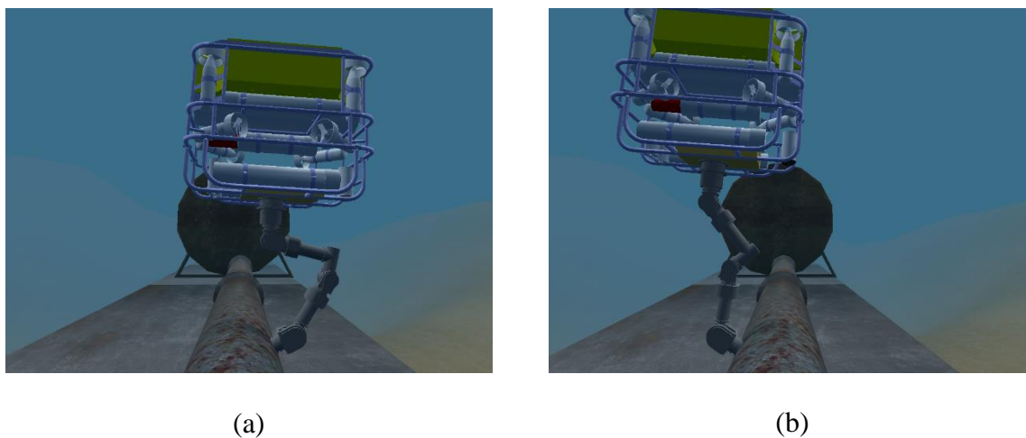
Figure 9: pipeline inspection simulation (a): starting position, (b) position at the end of the first movement In this case, we have simulated the execution of a free floating pipeline inspection task. We have considered a generalized version of the problem, where the end-effector is requested to follow a desired path, while maintaining a desired force whenever in contact with the pipeline surface. No a priori information of the pipeline's surface is exploited. Only the force and moments at the wrist are used to accomplish the task.
