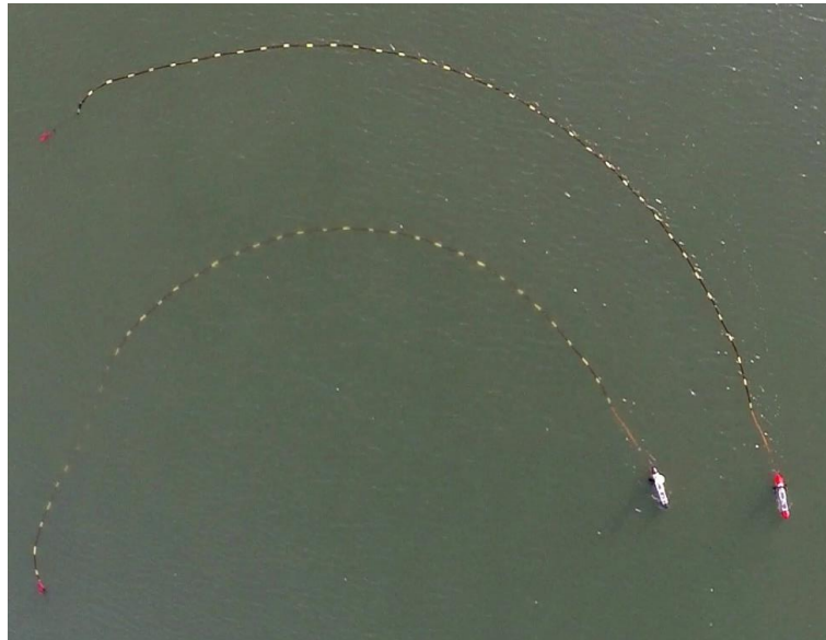
Fig. 7 Aerial view of two MEDUSA vehicles (IST) towing two streamers in a curve.
