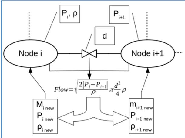
Figure 4. Calculation Process over all the Nodes
